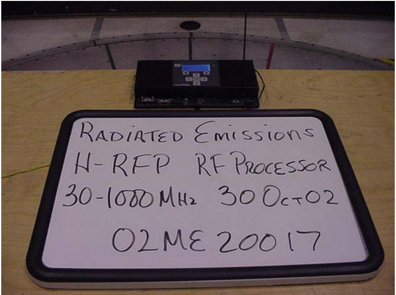
Radiated Emissions Test Set-Up 30-1000MHz (Model number in title block H-RFP = H-RFP-1P)
