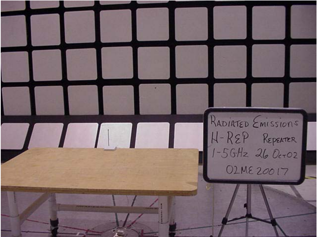
Radiated Emission Test Set-Up 1-5GHz Front View
