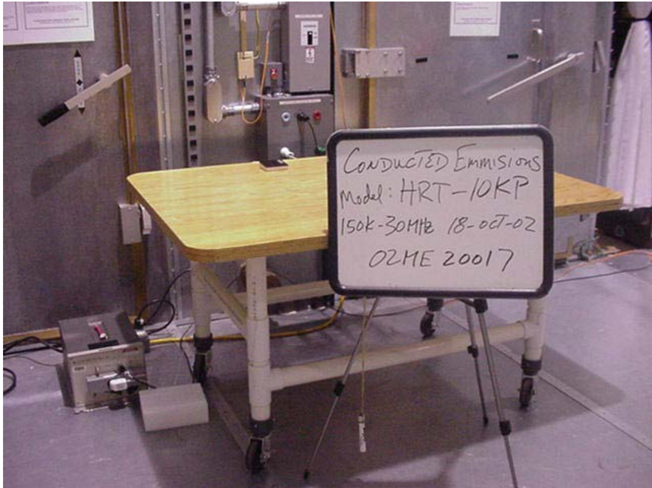
Conducted Emission Test Set-Up 0.150 to 30MHz
