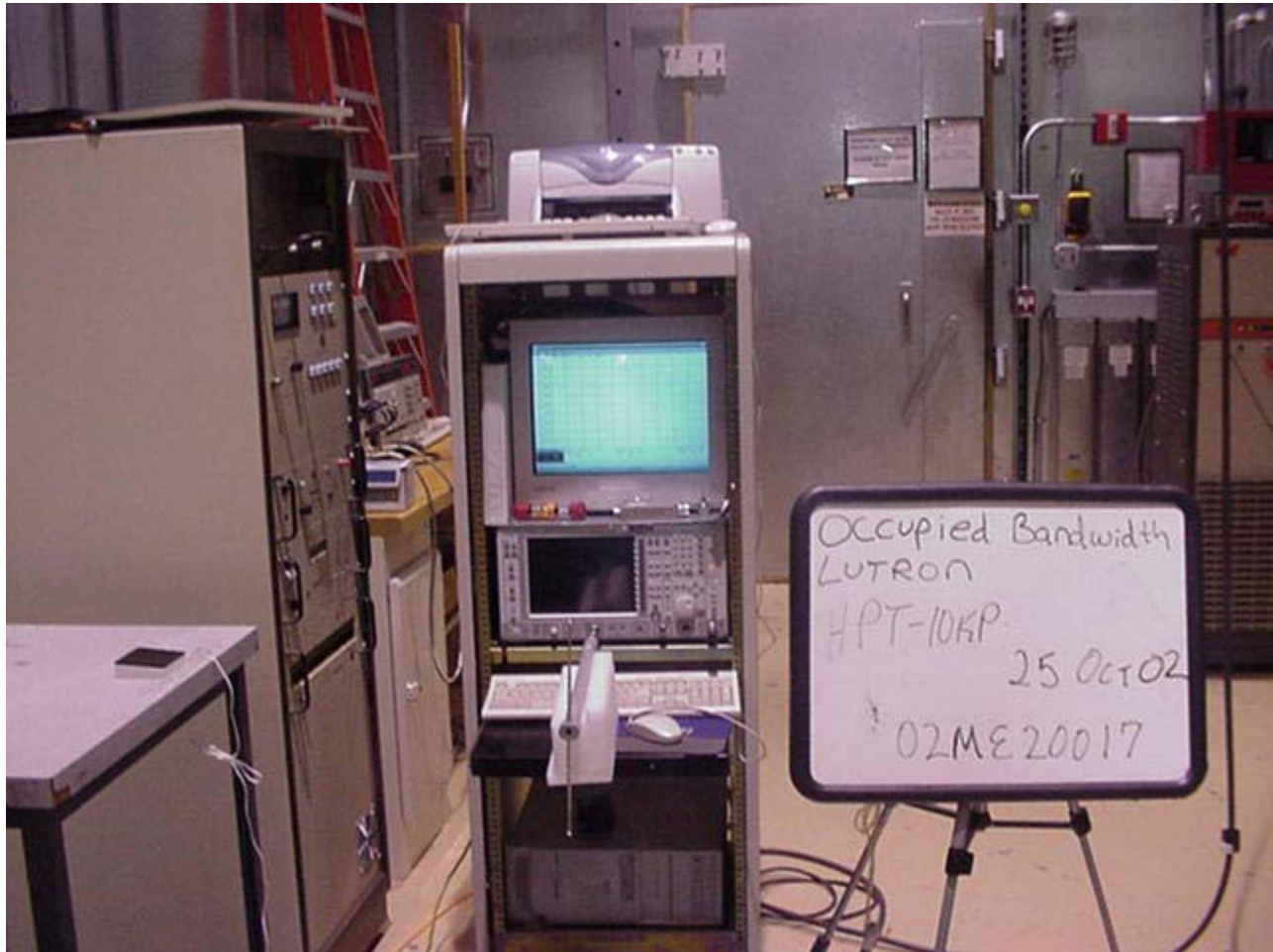
Occupied Bandwidth Test Set-Up HRT-10KP
