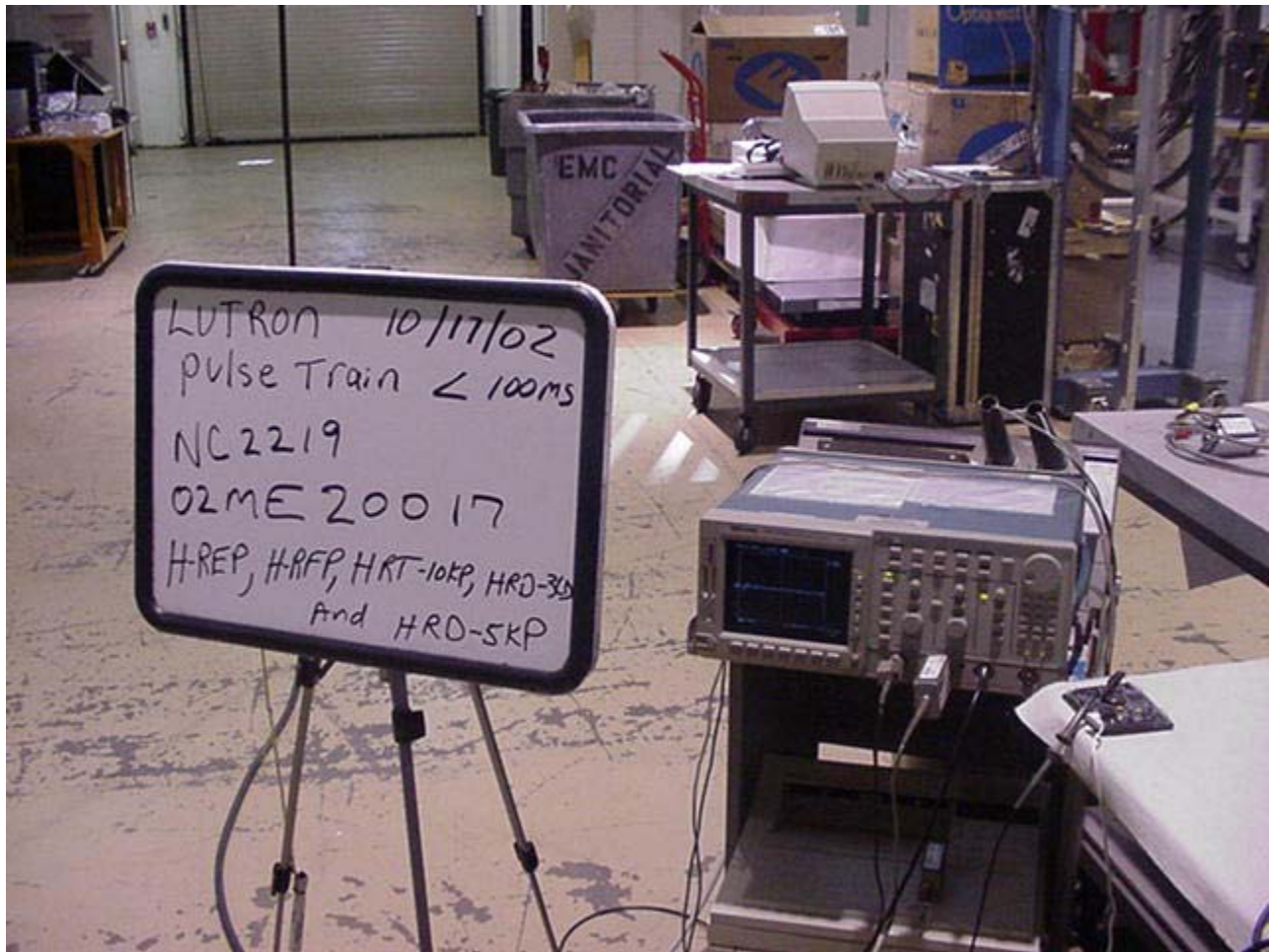
Pulse Train Test Set-Up
