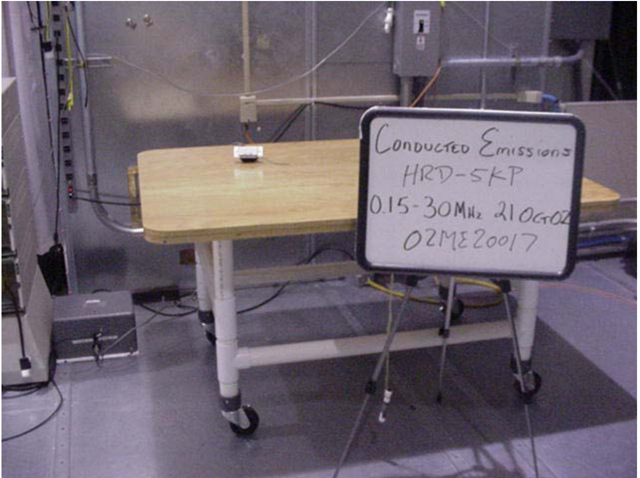
Conducted Emission Test Set-Up 0.150 to 30MHz
