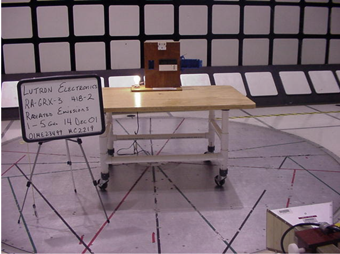
Radiated Emissions test 1 - 5GHz set-up
