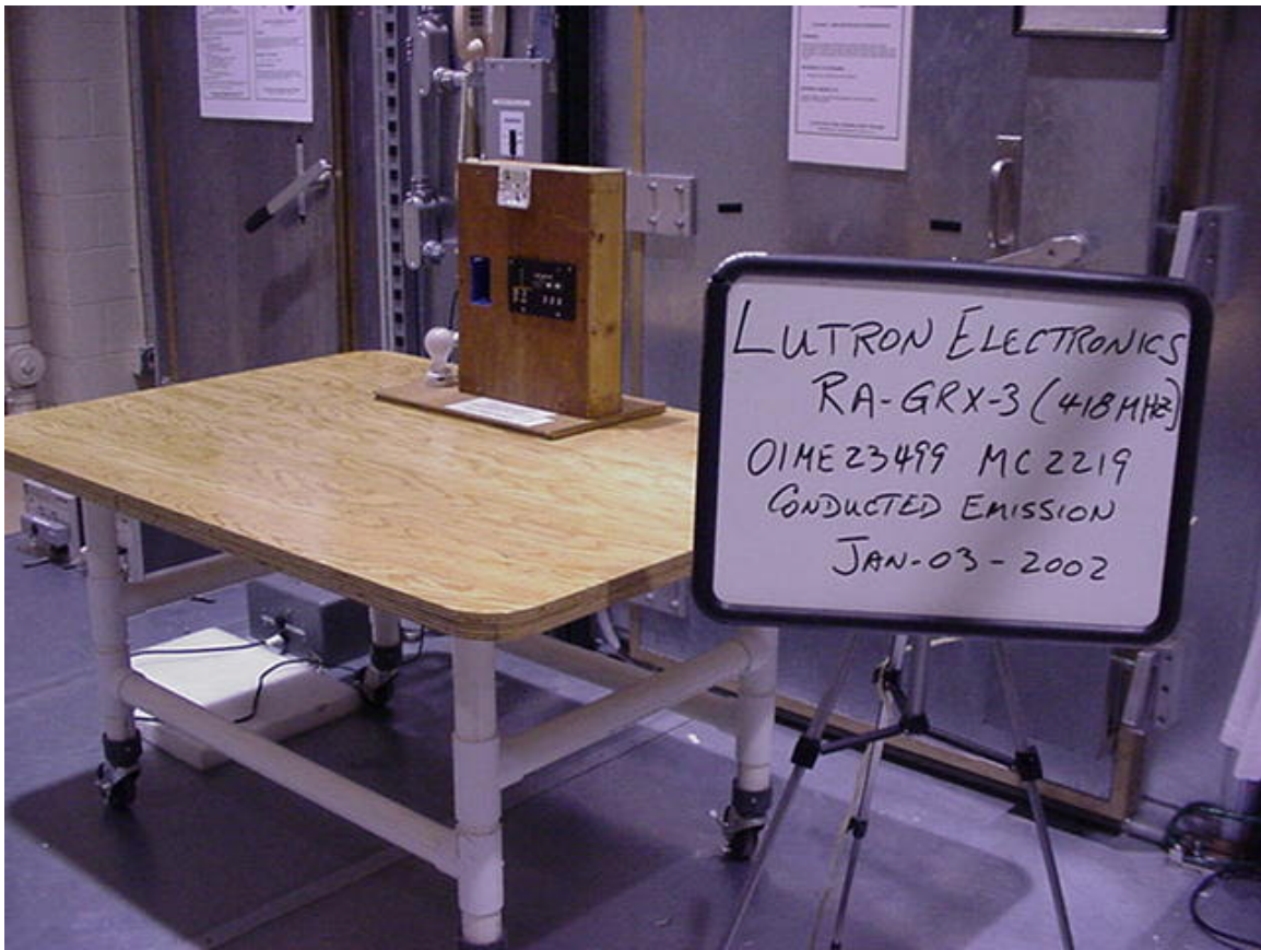
Conducted Emissions test set-up
