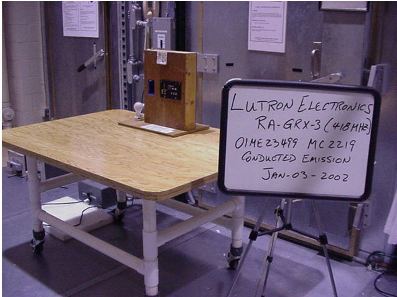
Conducted Emissions test set-up
