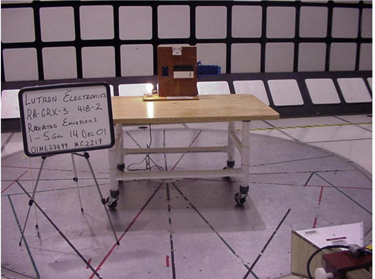
Radiated Emissions test 1 - 5GHz set-up
