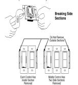
When removing side sections for multigang installations, reduction of the dimmers load capacity is required. See table below.
