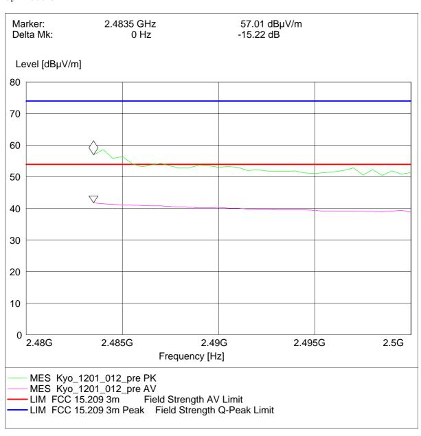
Radiated measurement (higher band edge)
