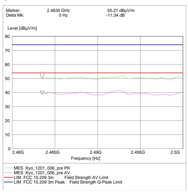
Radiated measurement (higher band edge)
