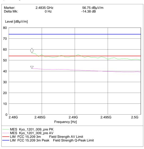
Radiated measurement (higher band edge)
