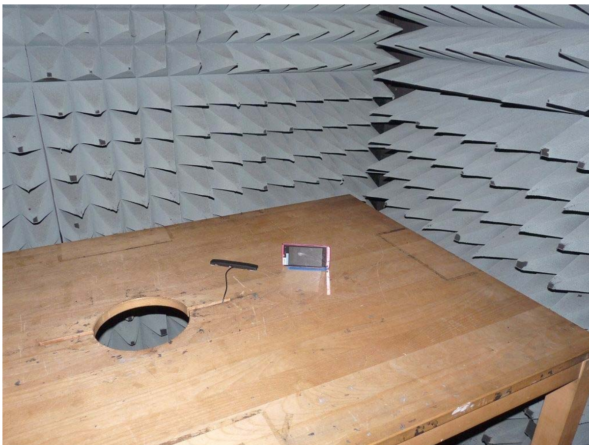
Photo 1: Test setup for radiated measurements (Enclosure, below 30 MHz, $15)
