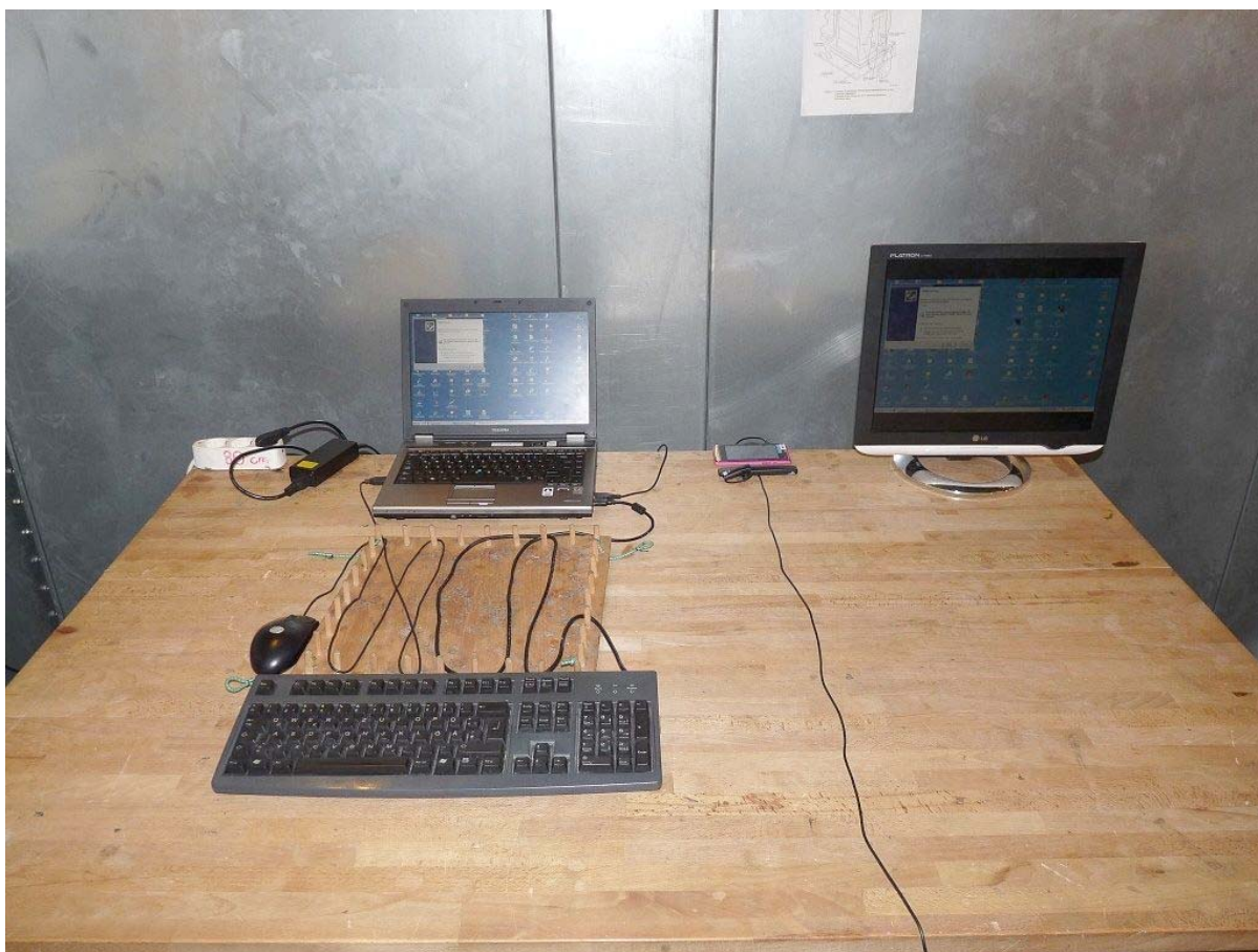
Photo 6: Test setup for conducted measurements (computer peripheral setup, EUT supplied by USB-cable from computer)
