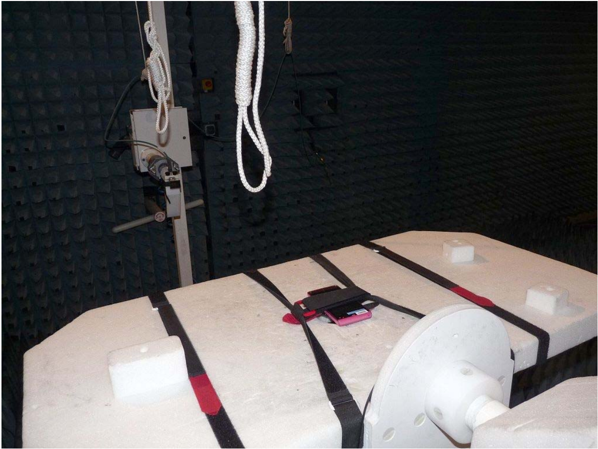
Photo 4: Test setup for radiated measurements (Enclosure, 18-25 GHz, § 15)
