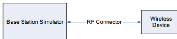
Figure 10.1 Power Measurement Setup
