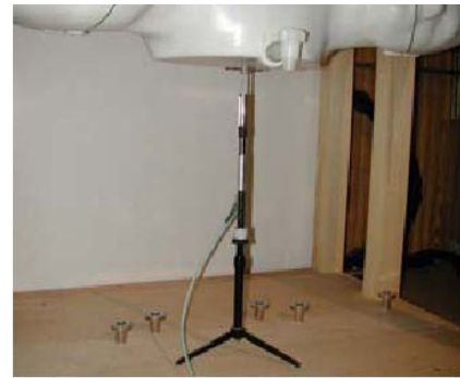
Figure 11.1 Dipole Verification Test Setup Diagram & Photo
