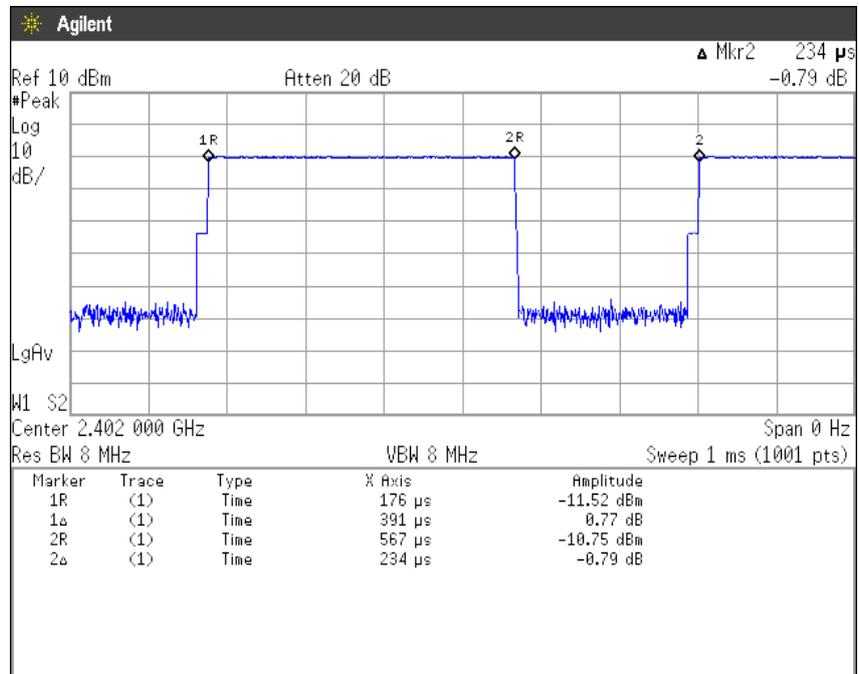
$$\text{Duty Cycle} = \text{Ton} / (\text{Ton} + \text{Toff}) = 391[\mu\text{s}] / (391[\mu\text{s}] + 234[\mu\text{s}]) = 62.56\%$$
