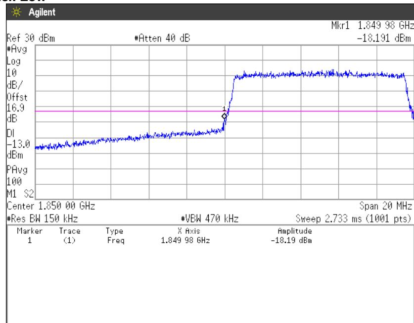
**16QAM, BW 10MHz, RB50-0****Channel: High**
