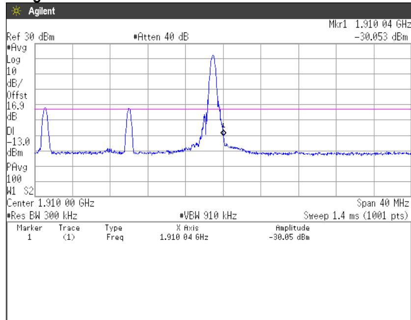
**QPSK, BW 20MHz, RB100-0****Channel: Low**
