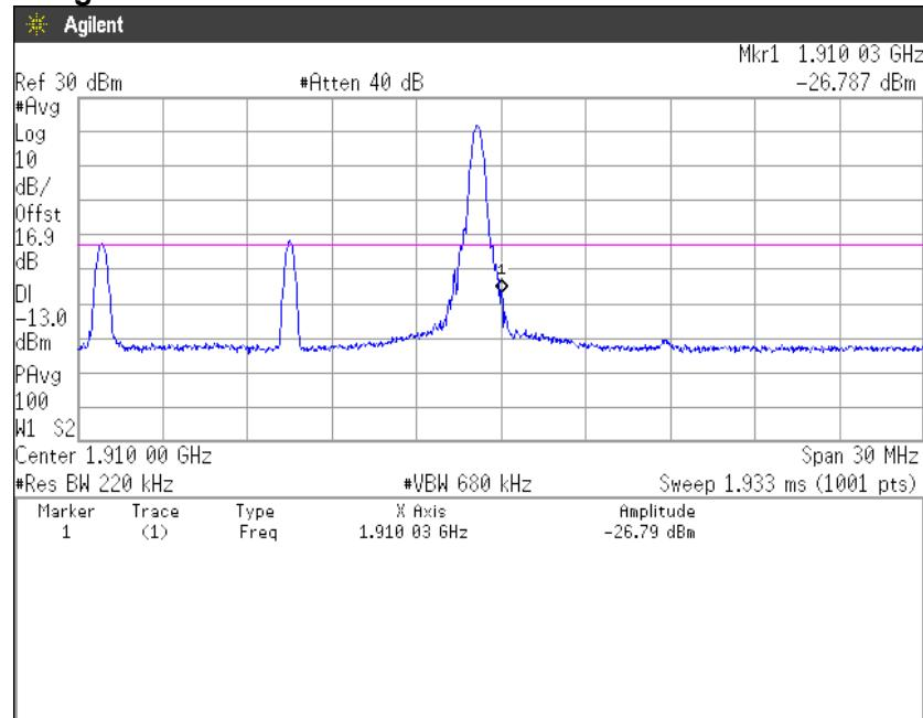
**16QAM, BW 15MHz, RB75-0****Channel: Low**
