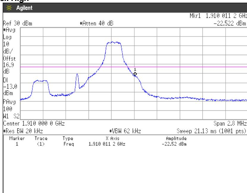
**QPSK, BW 1.4MHz, RB6-0****Channel: Low**
