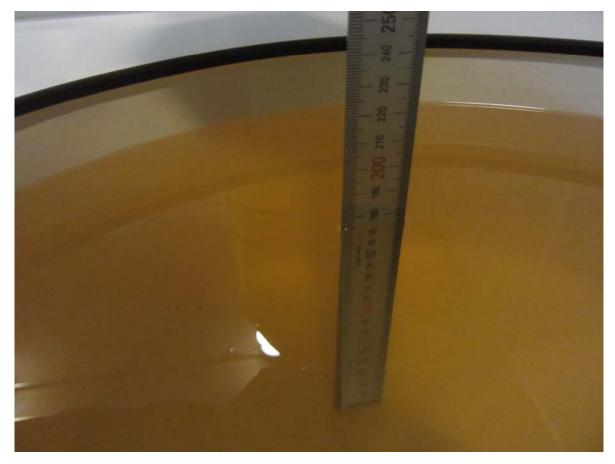
Note: The liquid depth is maintained at a minimum depth of 15 cm to minimize reflections from the upper surface.
