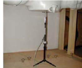
Figure 11.1 Dipole Verification Test Setup Diagram & Photo
