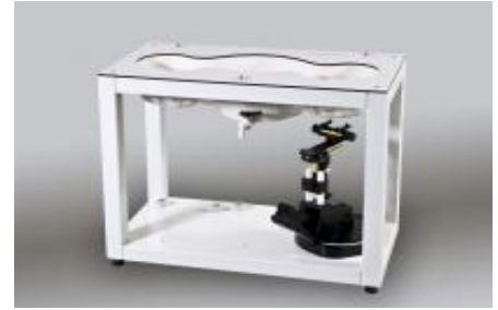
Figure 3.6 SAM Twin Phantom
