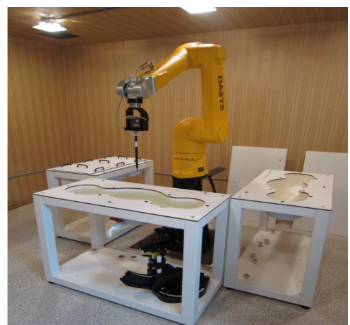
Figure 4.1 DASY5 Test System
