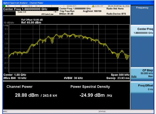
PAPR (dB) = P<sub>Pk</sub> (dBm) - P<sub>Avg</sub> (dBm) = 29.23 dBm - 28.88 dBm = 0.35 dB
