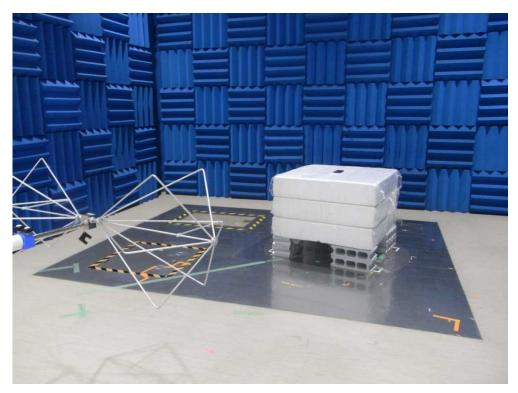
Radiated Emission for 300MHz to 1GHz
