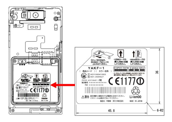
Note. The label location is inside the battery compartment. The label is attached to this device by an adhesive. The adhesive is permanent type with strong strength.
