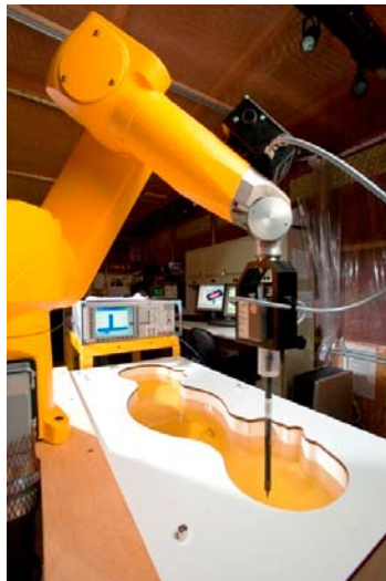
Figure 3-2 DASY4 SAR Measurement System
