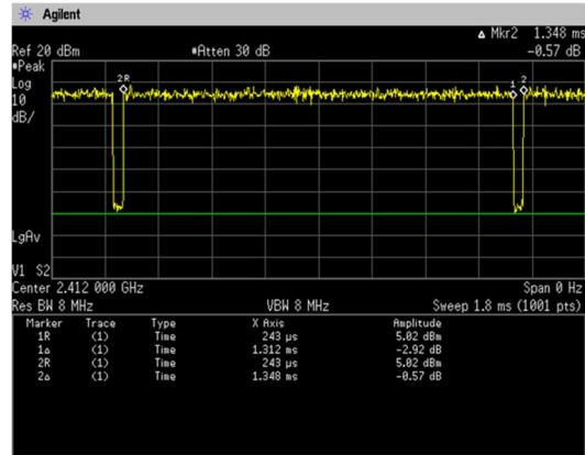
$$\text{Duty Cycle} = \text{Ton} / (\text{Ton} + \text{Toff}) = 1.312[\text{ms}] / (1.312[\text{ms}] + 0.036[\text{ms}]) = 97.33[\%]$$
