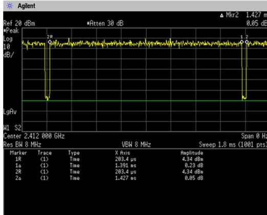
$$\text{Duty Cycle} = \text{Ton} / (\text{Ton} + \text{Toff}) = 1.391[\text{ms}] / (1.391[\text{ms}] + 0.036 [\text{ms}]) = 97.48[\%]$$
