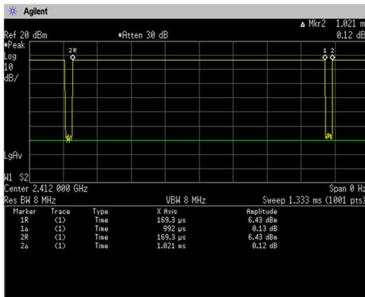
$$\text{Duty Cycle} = \text{Ton} / (\text{Ton} + \text{Toff}) = 0.992[\text{ms}] / (0.992[\text{ms}] + 0.029[\text{ms}]) = 97.16[\%]$$
