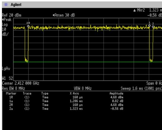
$$\text{Duty Cycle} = \text{Ton} / (\text{Ton} + \text{Toff}) = 1.286[\text{ms}] / (1.286[\text{ms}] + 0.037[\text{ms}]) = 97.2[\%]$$
