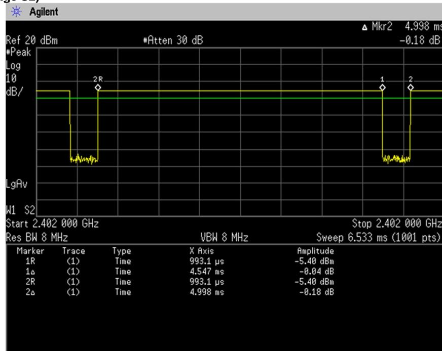
$$\text{Duty Cycle} = \text{Ton} / (\text{Ton} + \text{Toff}) = 4.547[\text{ms}] / (4.547[\text{ms}] + 0.451[\text{ms}]) = 90.98[\%]$$
