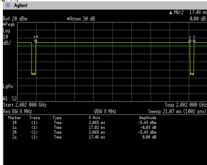
$$\text{Duty Cycle} = \text{Ton} / (\text{Ton} + \text{Toff}) = 17.02[\text{ms}] / (17.02[\text{ms}] + 0.44[\text{ms}]) = 97.48[\%]$$
