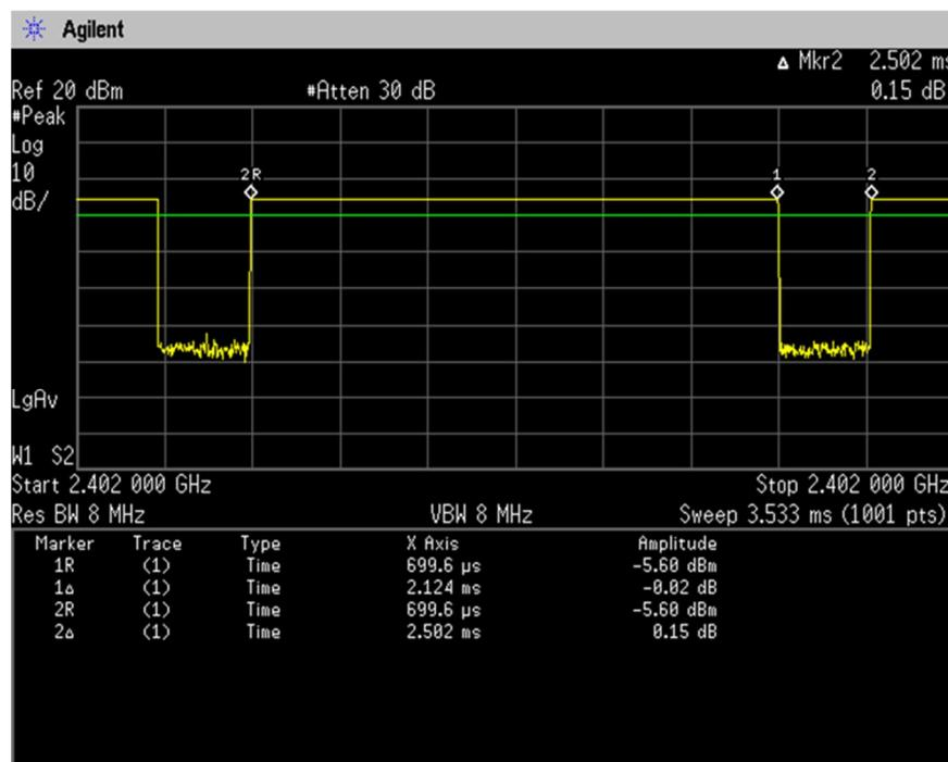
$$\text{Duty Cycle} = \text{Ton} / (\text{Ton} + \text{Toff}) = 2.124[\text{ms}] / (2.124[\text{ms}] + 0.378[\text{ms}]) = 84.89[\%]$$
