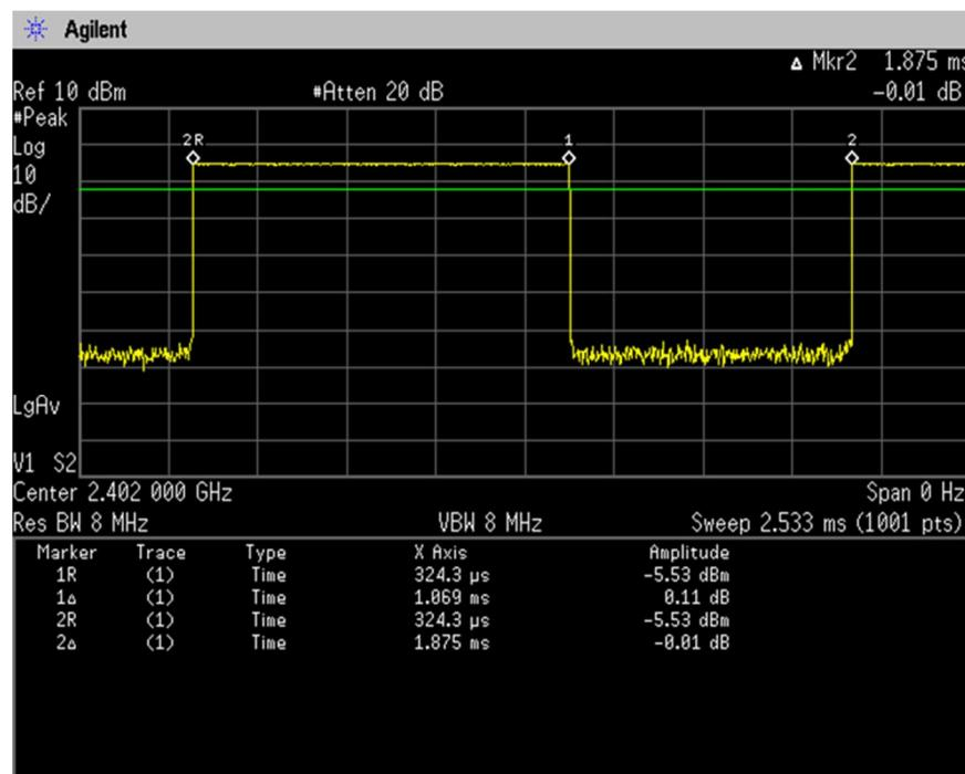
$$\text{Duty Cycle} = \text{Ton} / (\text{Ton} + \text{Toff}) = 1.069[\text{ms}] / (1.069[\text{ms}] + 0.806[\text{ms}]) = 57.01[\%]$$
