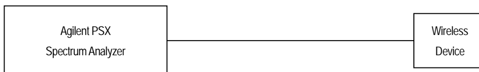
Figure 10.5 Power Measurement Setup for Bandwidths > 50 MHz
