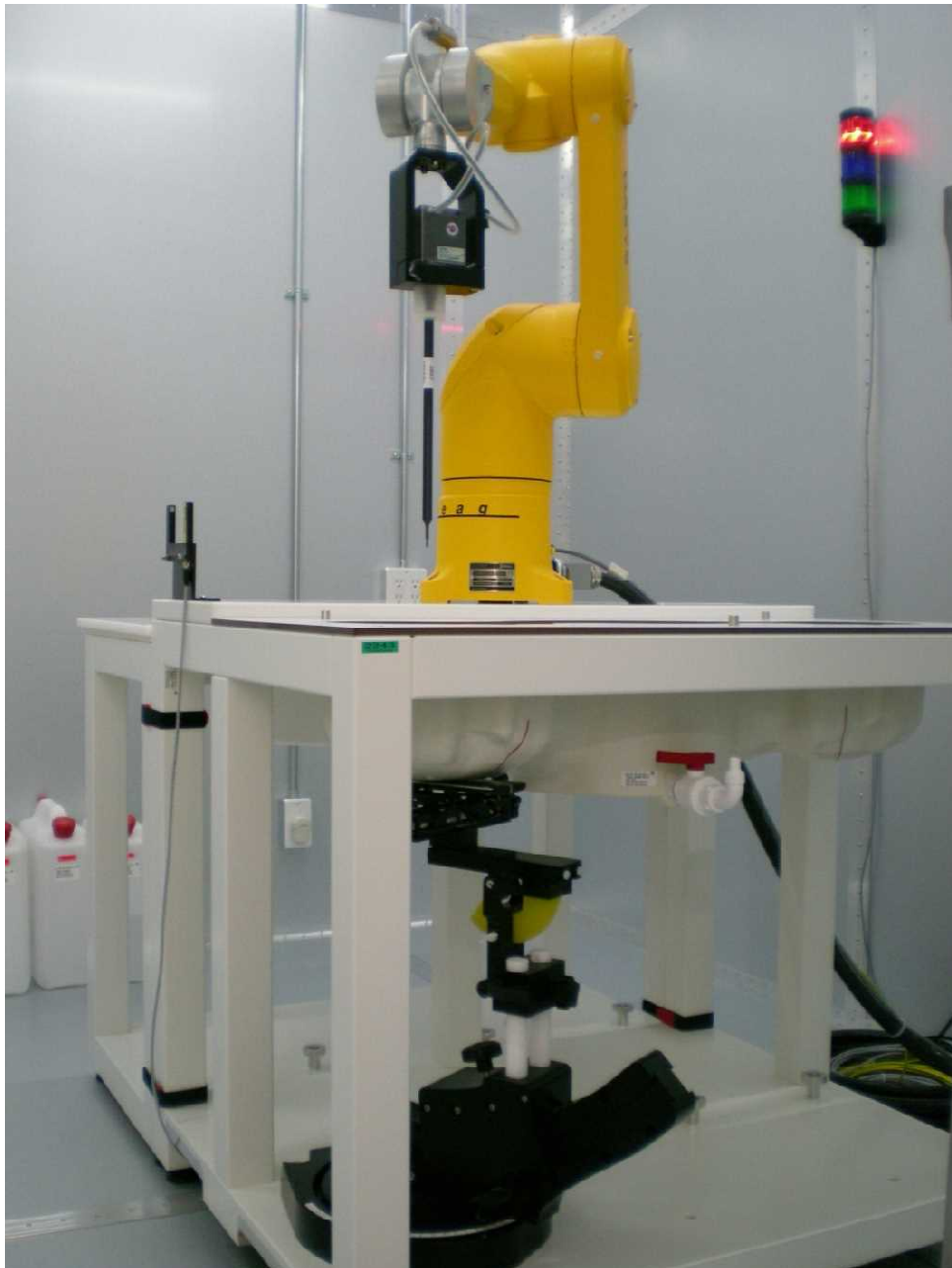
Test setup photo(Head SAR Test photo)
