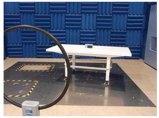
Transmitter Radiated Spurious Emissions (RF Radiated test)
