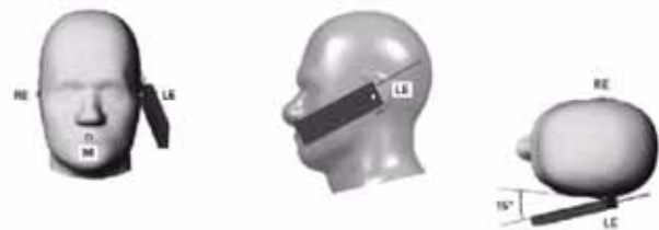
Figure 7.3 Front, Side and Top View of Ear/15° Position
