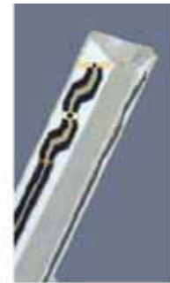
Figure 3.3 Probe Thick-Film Technique
