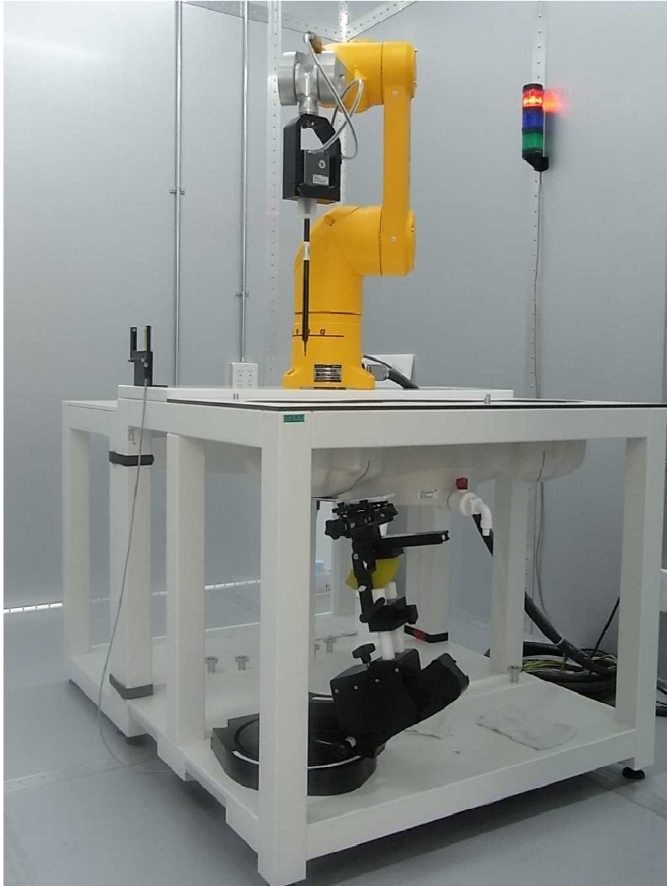
Test setup photo(Head SAR Test photo)
