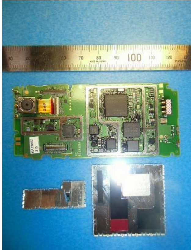
Main PCB L8 without shield
