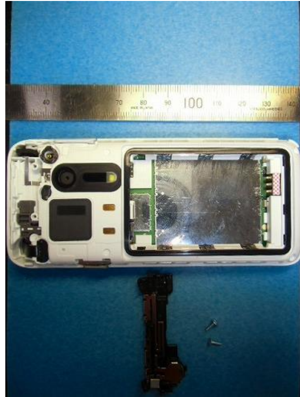
KEY REAR open & Main Antenna
