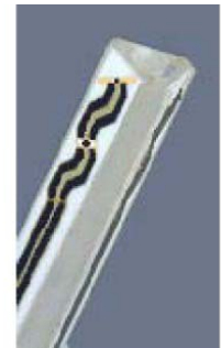
Figure 3.3 Probe Thick-Film Technique
