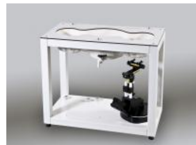
Figure 3.6 SAM Twin Phantom
