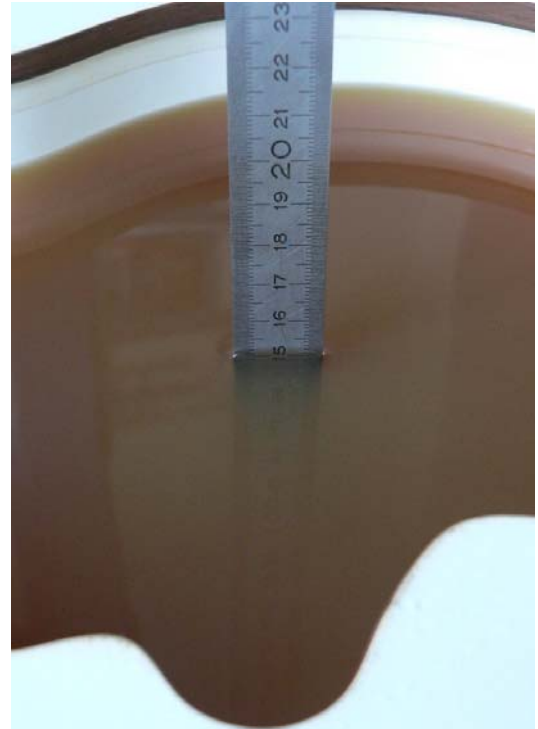
Fig. 49: Liquid depth for IEEE 802.11 a, head measurements
