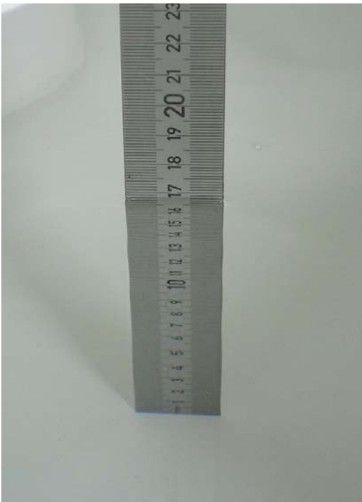
Fig. 50: Liquid depth for IEEE 802.11 b/g, body measurements
