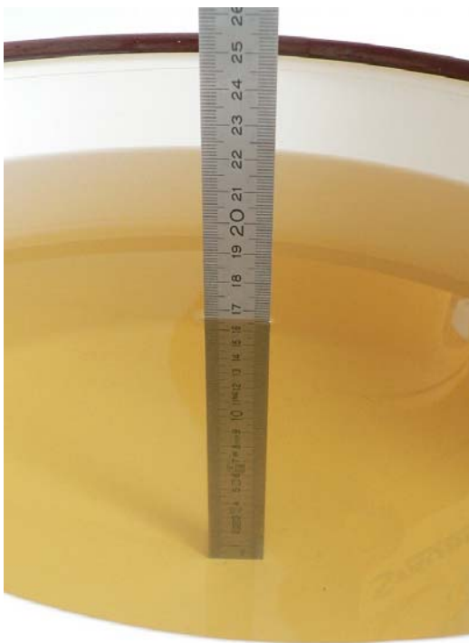
Fig. 46: Liquid depth for GSM/GPRS 850 and CDMA 2000, body measurements.
