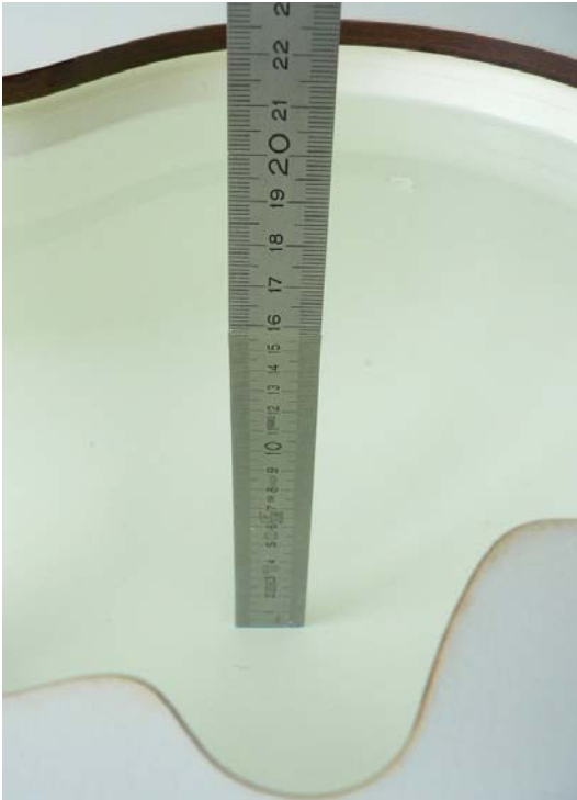
Fig. 48: Liquid depth for IEEE 802.11 b/g, head measurements
