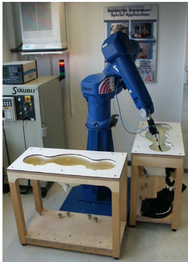
Fig. 7: The measurement set-up with two SAM phantoms containing tissue simulating liquid.
