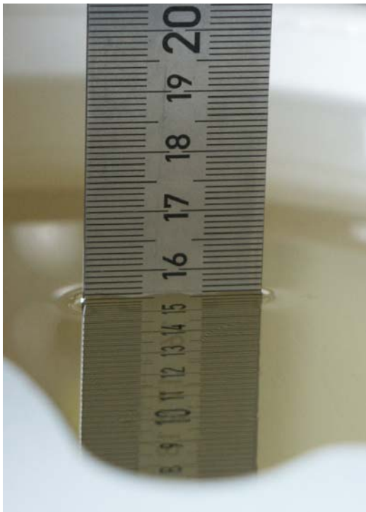
Fig. 44: Liquid depth for GSM/GPRS 850, WCDMA V and CDMA 2000, head measurements
