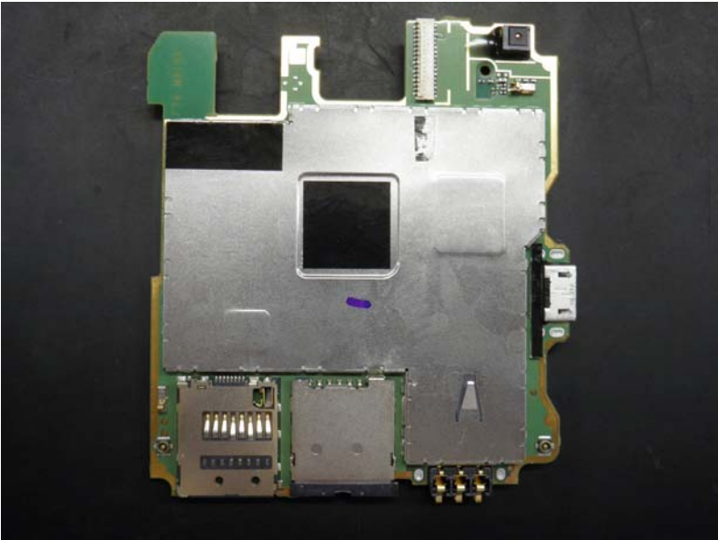
MAIN PCB L1 with shield
