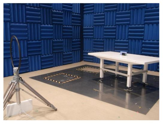
Radiated Emission for 30MHz to 300MHz
