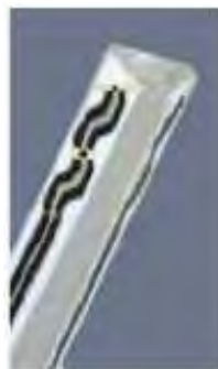
Figure 4.3 Probe Thick-Film Technique
