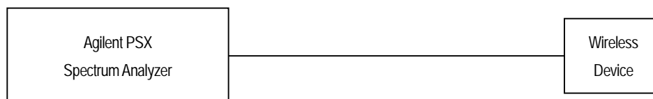
Figure 10.5 Power Measurement Setup for Bandwidths > 50 MHz
