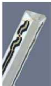
Figure 4.3 Probe Thick-Film Technique
