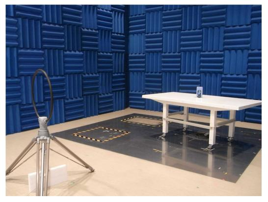
Radiated Emission for 30MHz to 300MHz
