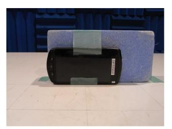
Note: X-axis generates the maximum emission at Bluetooth, GSM1900 and WCDMA Band II Y-axis generates the maximum emission at NFC.
