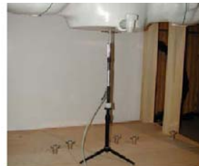
Figure 11.1 Dipole Verification Test Setup
