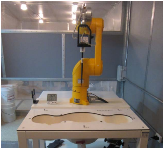
Figure 2.2 DASY5 Test System
