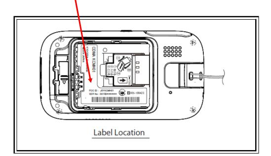
The label is attached to this device by an adhesive. The adhesive is permanent type with strong strength. Additionally, the label is readily to the purchaser at the time of purchase.
