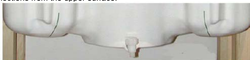
Figure 5.1 Sam Twin Phantom shell
