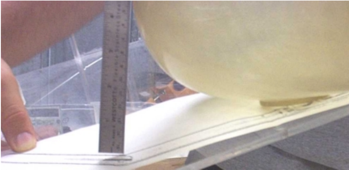
Figure 8. Side View of IDX Phantom with 2-Dimensional Phone Simulation (add 3cm).
