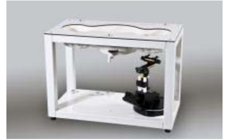
Figure F.5.1 SAM Twin Phantom
