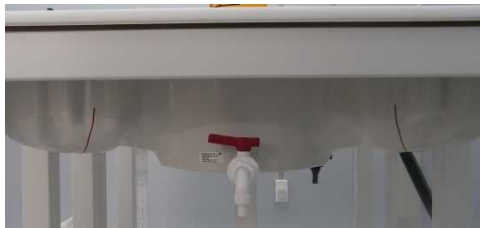
Figure 4.6 SAM Twin phantom
