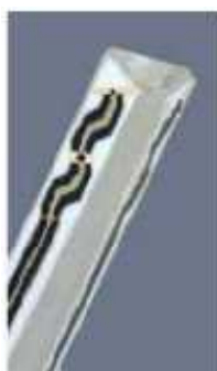
Figure 4.3 Probe Thick-Film Technique
