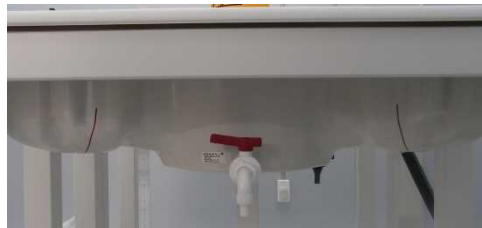
Figure 4.6 SAM Twin phantom
