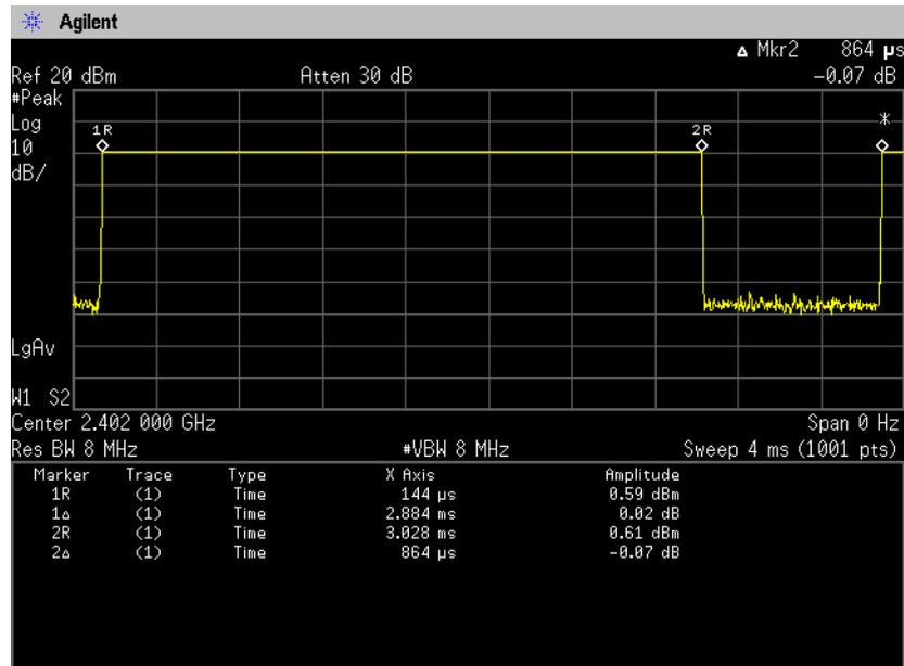
$$\text{Duty Cycle} = T_{\text{on}} / (T_{\text{on}} + T_{\text{off}}) = 2884[\mu\text{s}] / (2884[\mu\text{s}] + 864[\mu\text{s}]) = 77.0[\%]$$
