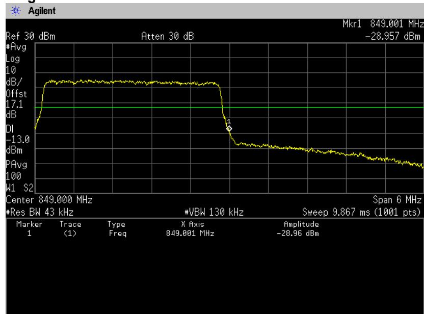
**16QAM, BW 3MHz, RB1-0****Channel: Low**
