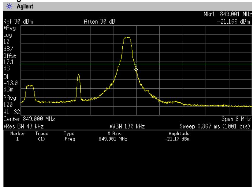
**QPSK, BW 3MHz, RB15-0****Channel: Low**
