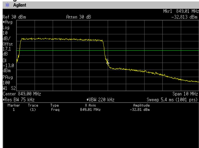
**QPSK, BW 10MHz, RB1-0****Channel: Low**
