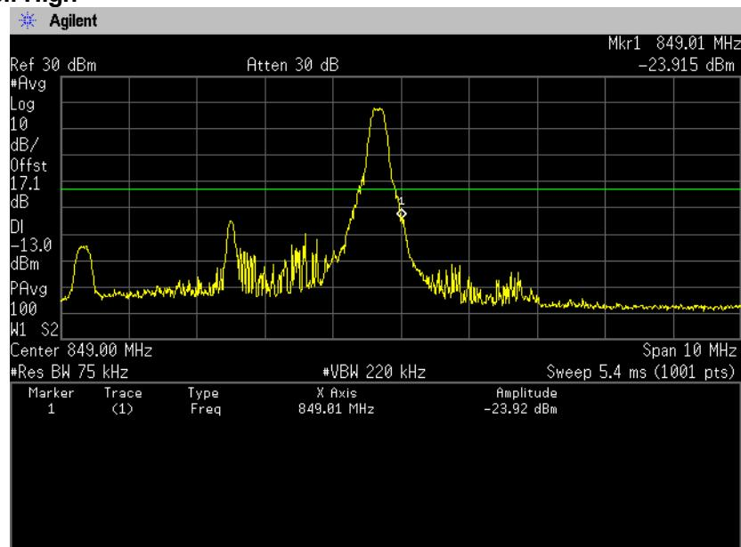
**16QAM, BW 5MHz, RB25-0****Channel: Low**
