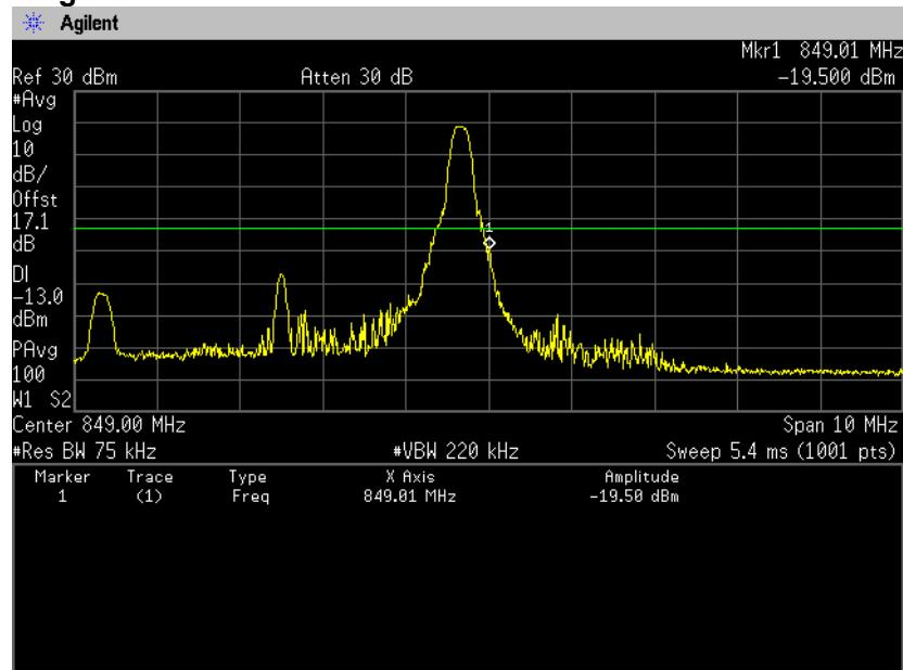
**QPSK, BW 5MHz, RB25-0****Channel: Low**
