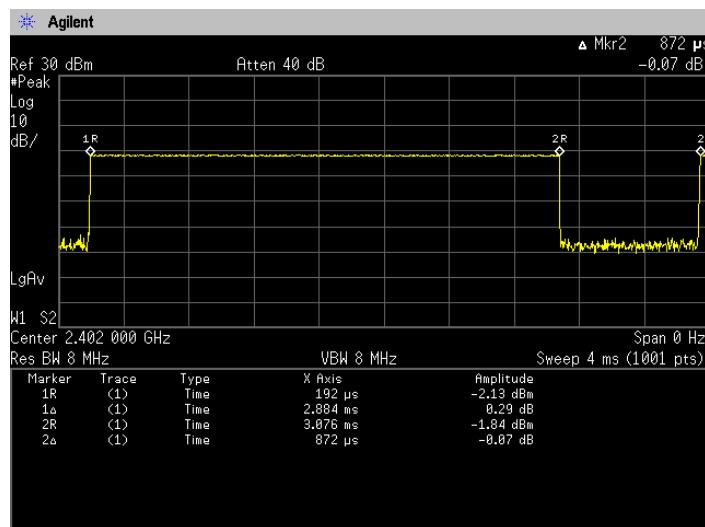
$$\text{Duty Cycle} = T_{\text{on}} / (T_{\text{on}} + T_{\text{off}}) = 2884[\mu\text{s}] / (2884[\mu\text{s}] + 872[\mu\text{s}]) = 76.8[\%]$$
