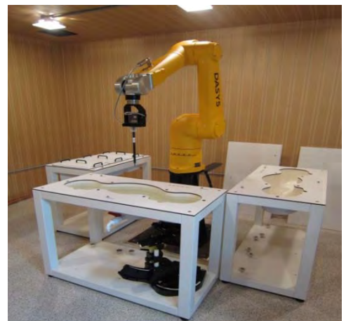
Figure E.7.1 DASY5 Test System
