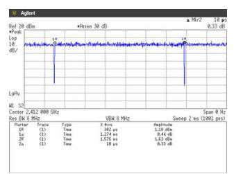
Duty Cycle = Ton / (Ton + Toff) =  $1274[\mu s] / (1274[\mu s] + 10[\mu s]) = 99.22[\%]$
