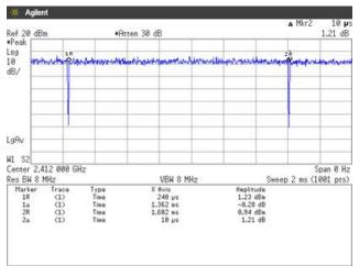
Duty Cycle =  $Ton / (Ton + Toff) = 1362[\mu s] / (1362[\mu s] + 10[\mu s]) = 99.27[%]$
