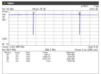
Duty Cycle =  $Ton / (Ton + Toff) = 1024[\mu s] / (1024[\mu s] + 8[\mu s]) = 99.22[\%]$
