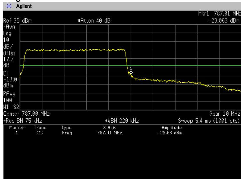
**16QAM, BW 5MHz, RB1-0****Channel: Low**
