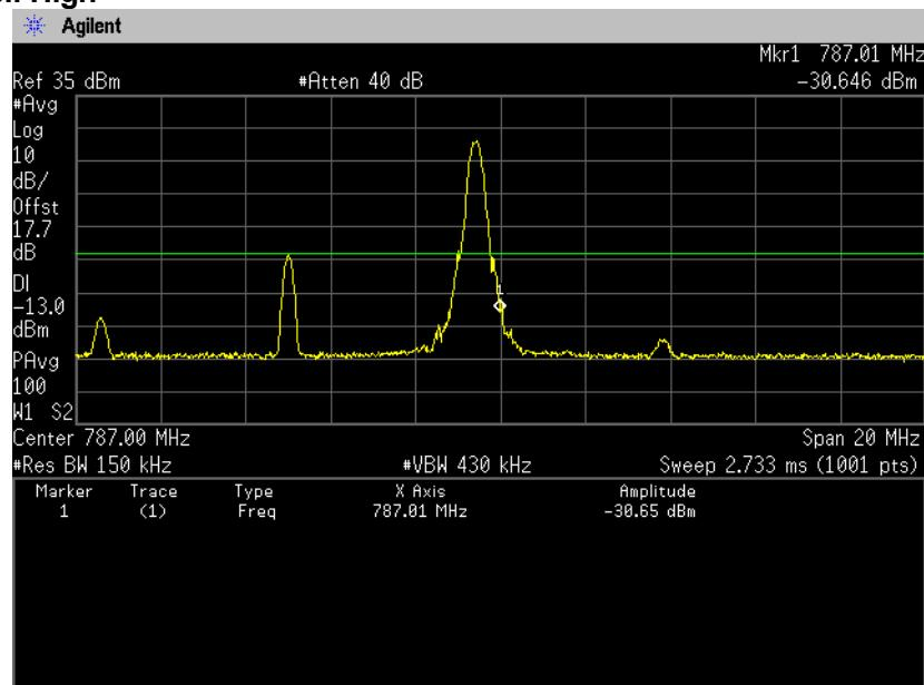
**16QAM, BW 10MHz, RB50-0****Channel: Low**
