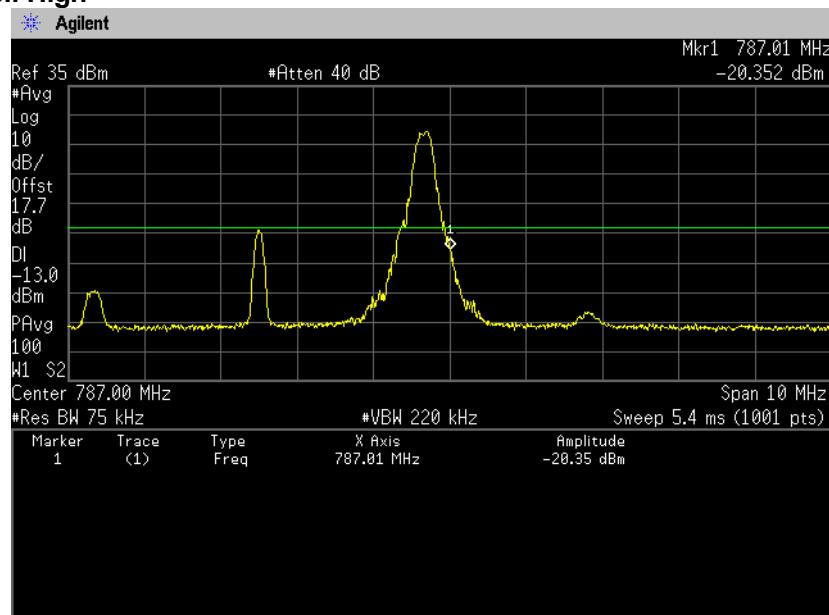
**16QAM, BW 5MHz, RB25-0****Channel: Low**
