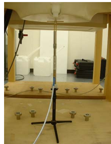
1800MHz System performance check setup
